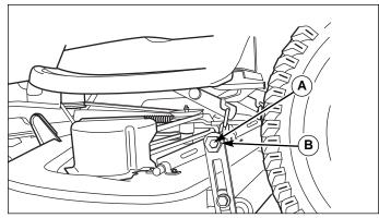
Figure 8. Leveling The Mower Side-to-Side Eccentric Nut Models
